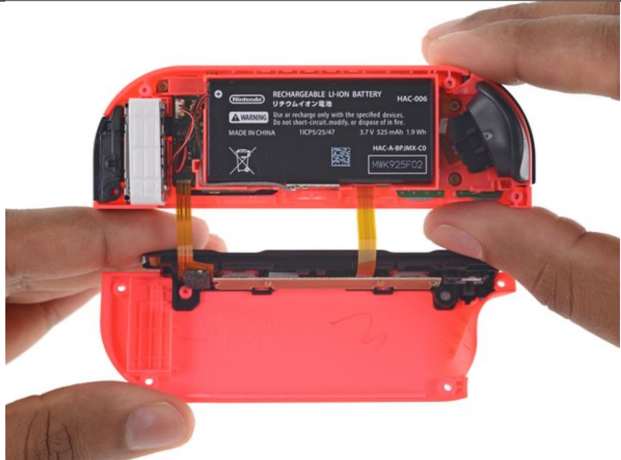
Photograph of Switch handheld controller showing LRA at left ( https://www.ifixit.com/Teardown/Nintendo+Switch+Teardown/78263 ).
